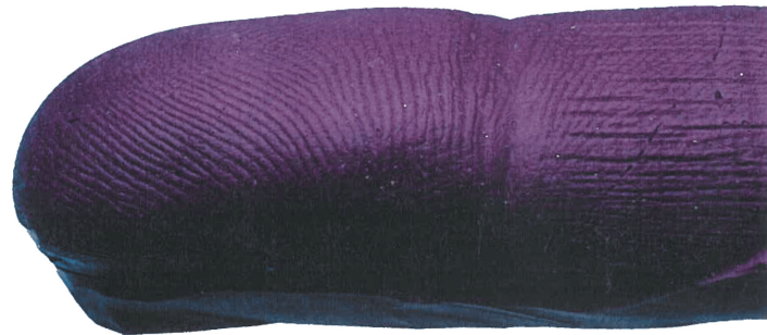
Artificial Finger to Evaluate Touch of Fabric (Source: S. S. Ramkumar, Ph.D. Work, 1998, University of Leeds, UK)
