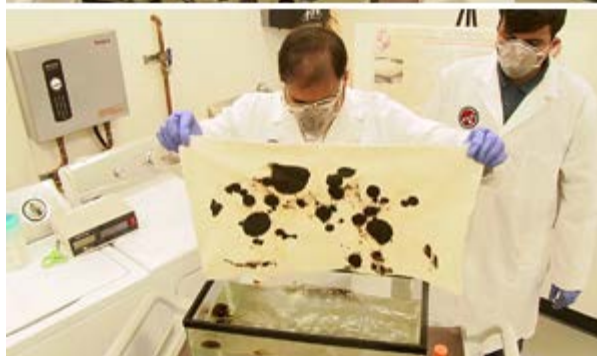
Texas Tech researchers take batting made from raw cotton (top) and lay it atop spilled oil floating on water. When they remove it again (bottom), the oil has left the water and now clings to the batting.
