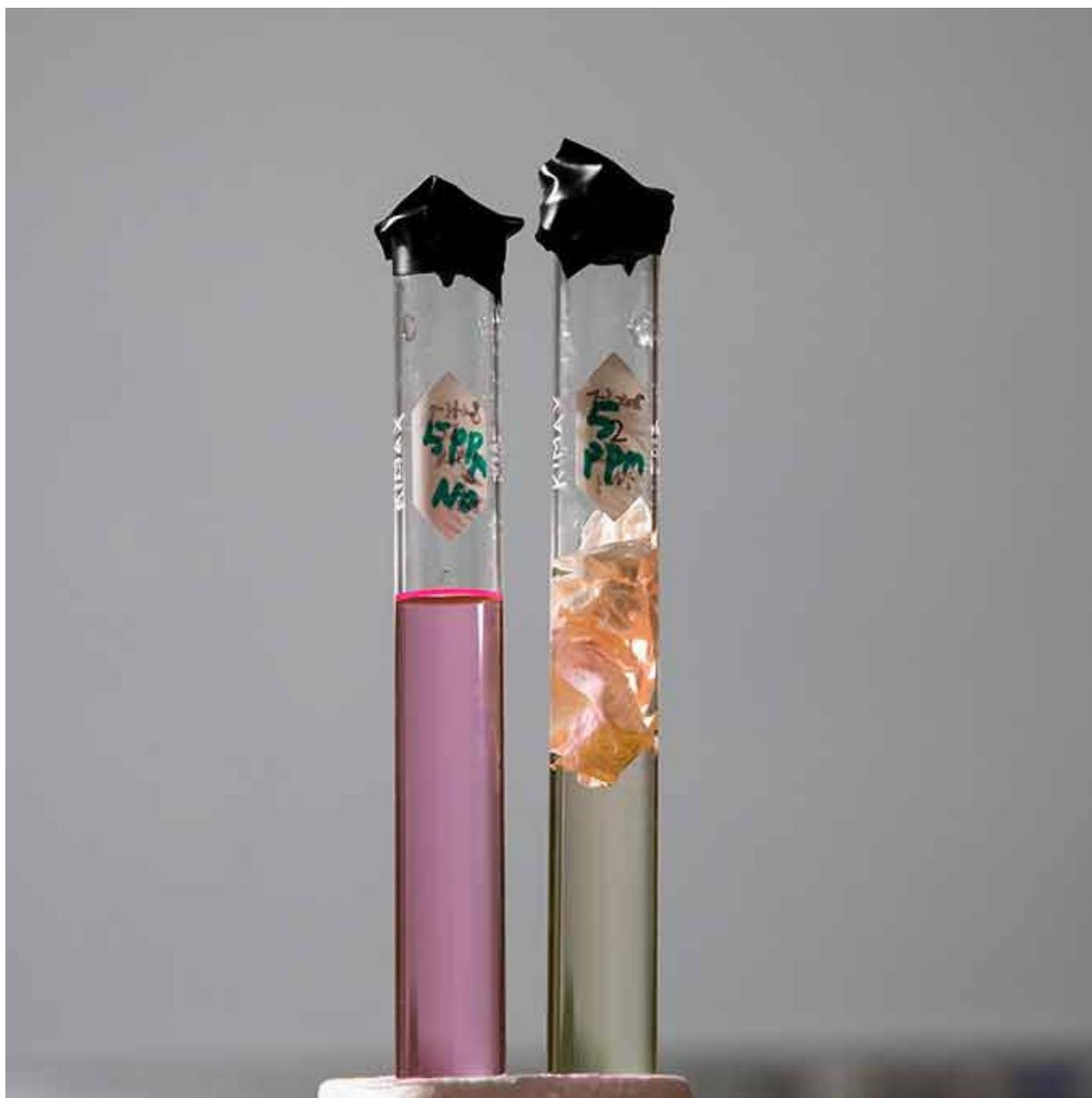
The tube on the left shows a red dye solution. In the tube on the right, the dye was trapped by a reusable web invented by a team at Texas Tech University. Light can then break down the dye.
